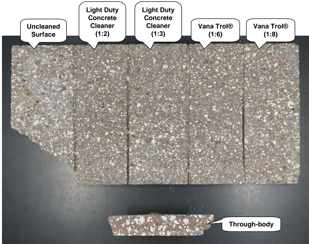
"Mountain Brown" Ground Face CMU After Cleaning
